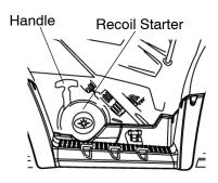
**NOTE:** The rope will be harder to pull when the engine is on a compression stroke. When a compression stroke is found, continue pulling the rope just until the engine rolls past the stroke, then stop pulling immediately.
